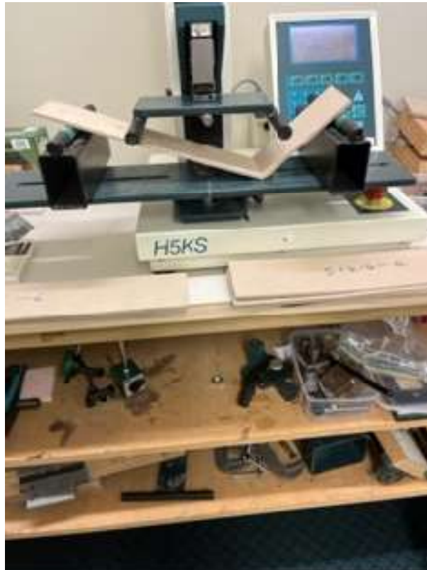
Figure 6 - 4pt Flex testing for new specimens
